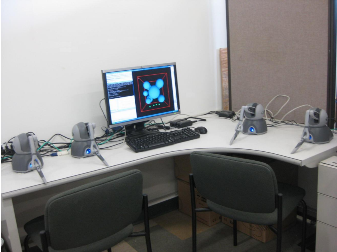
Figure 1. The complete experimental setup during the experiments. In this photo, the sphere interaction simulation has just begun, and all four Omnis are activated and are seen “hovering” above the table as they are in fact resting on the “floor” of the virtual environment. The subjects sit in the chairs and each control two of the Omnis during this practice trial. During the materials analysis experiment, the two subjects control only the left two Omnis, the third acts as the slave robot and actually interacts with the materials, and the fourth is deactivated.
